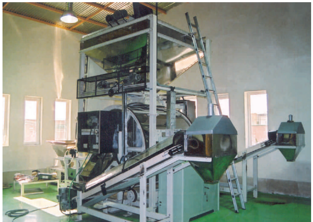
Single 500 kg Flavouring Drum with Storage Hopper 200 kg Flavouring Drum also available
