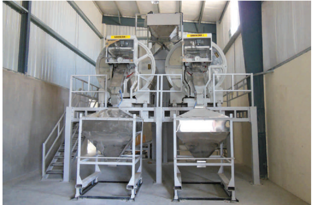
Dual Tea flavouring drum 500 kg capacity
