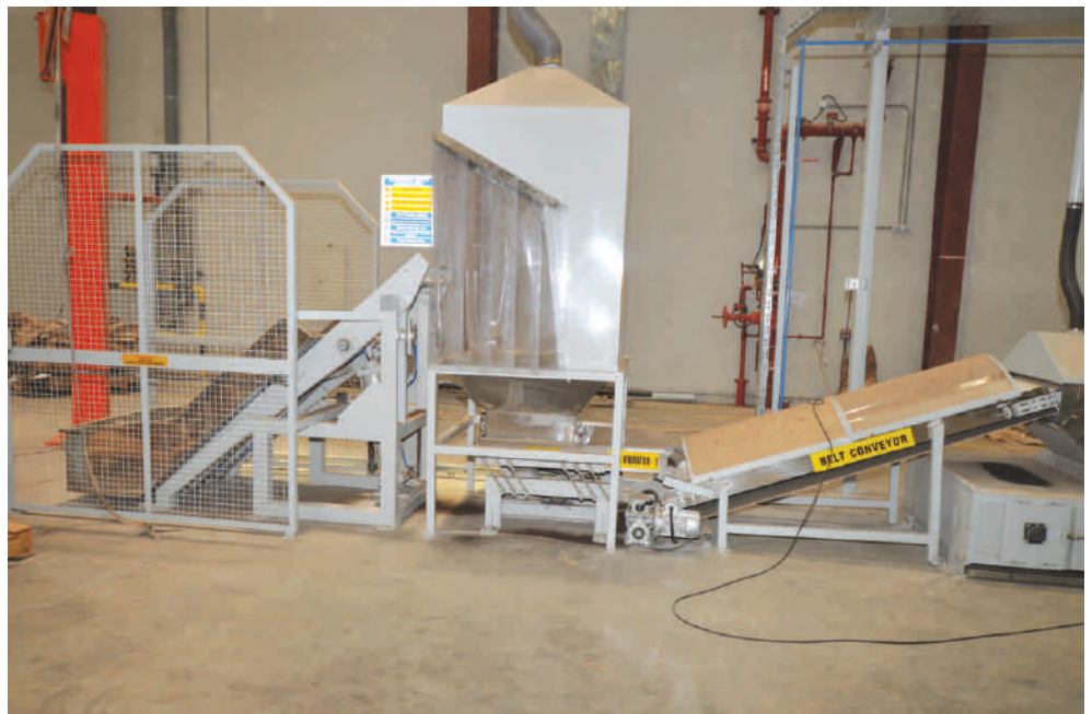
Pneumatic loose Tea feeding arrangement.
