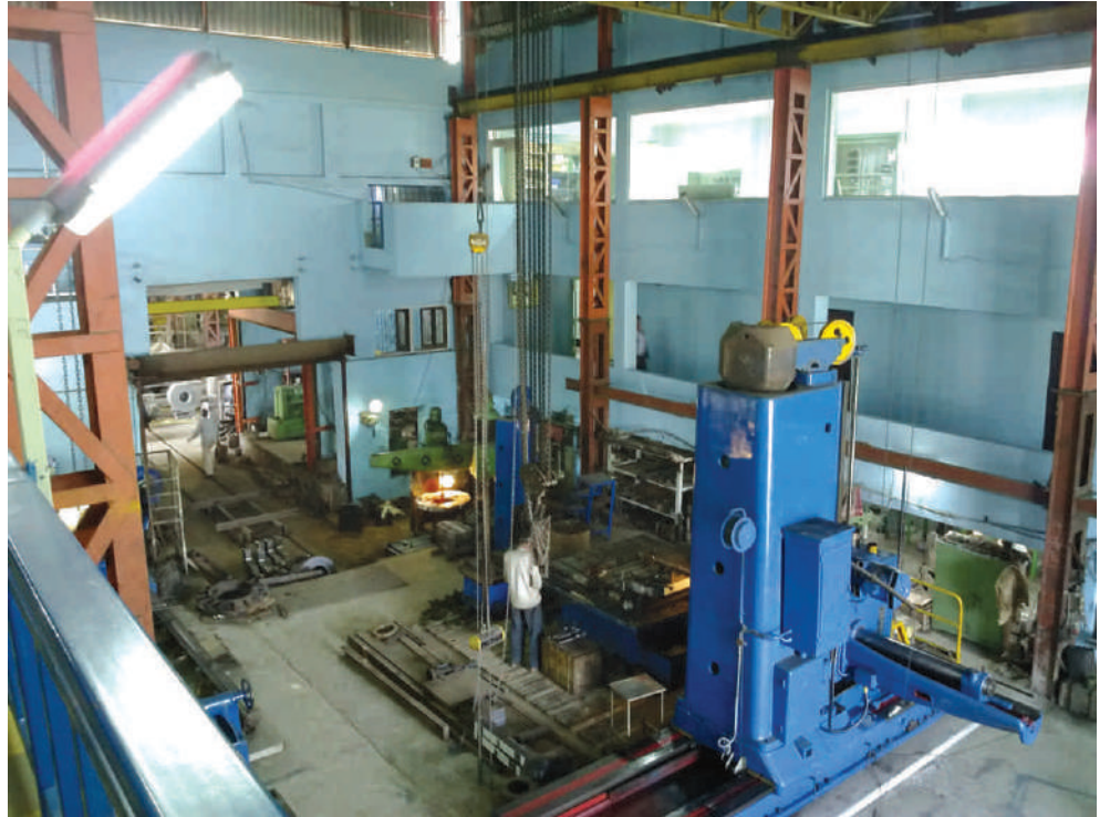
160 Spindle Dia Boring Maching for heavy engineering
