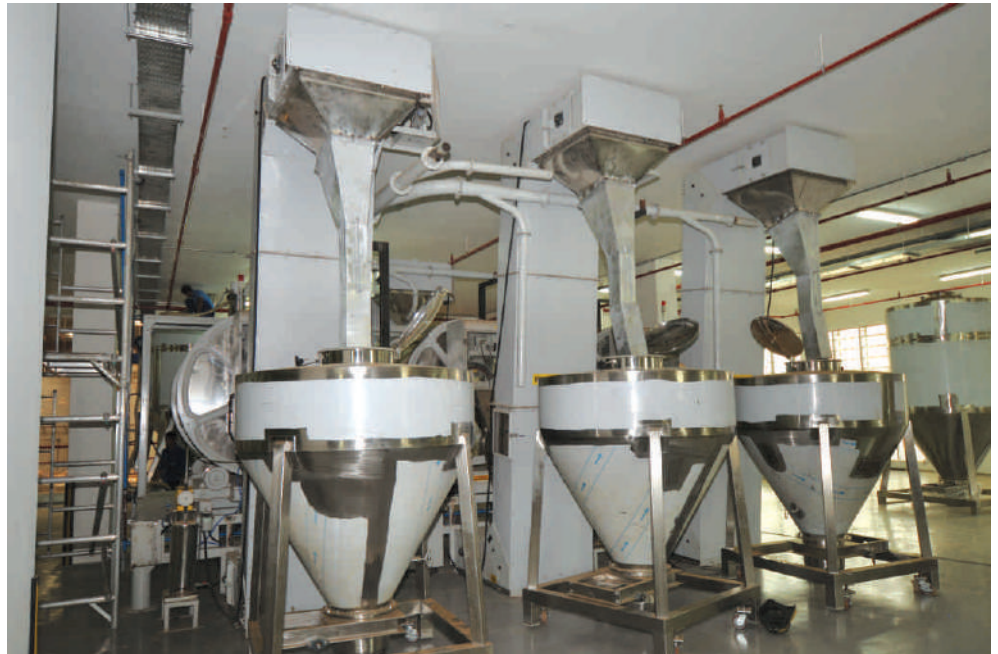
Mobile Hopper loading station on the Mezzanine Floor.
